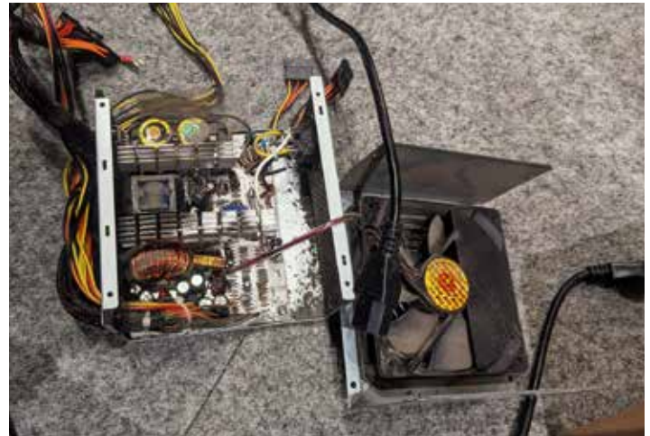
Above: The OC&E layout had originally used Personal Computer power supplies to supply 5-volt and 12-volt DC power to the SMINIs and Tortoise by Circuitron switch motors. They are great for collecting dirt and will eventually fail when the fans become clogged. Below Left: Bob Pilk is lining Track 4 and fastening the track to the roadbed with clear adhesive. Below Right: Tim Frade watches Darrel Ellis finish wiring one of the switch motors. This was a great opportunity to transfer some of the knowledge that our expert volunteers have accumulated over the years.
