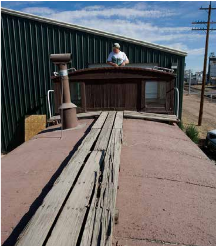
Above left: The running boards are all rotted out. The roof appears to be a very dull red faded tar paper over tongue and groove wood, supported by curved carlins. The Colorado weather is hard on cars of wood construction, so inside storage is essential for 10583's long term health..
