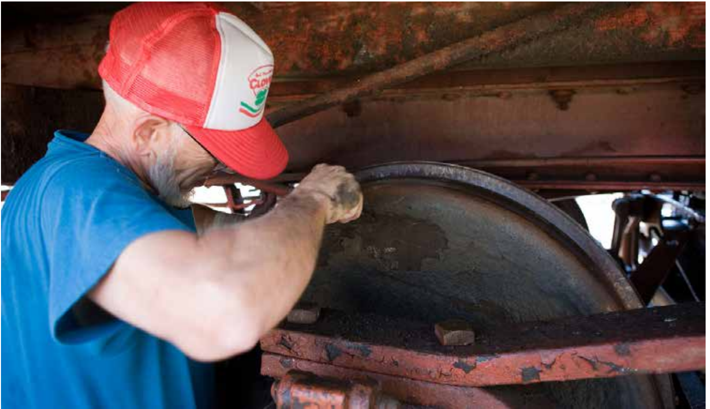
Above: John Keyser scrapes the remaining grease off of each wheel. Railway Preservationists often debate whether displayed equipment should be restored to a “new” condition, or maybe a “typical use” condition. Since our museum visitors are normally not “railfans”, we didn’t want to explain why the car looked dirty and dingy. Below: The caboose is pushed back into the museum building. Both Photos by Bob Sobol
