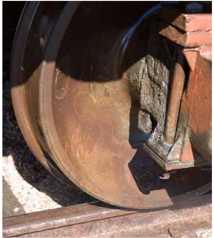
Above right: This wheel reveals some unusual symmetrical round welds and a number of marks that were hidden under decades of journal grease. We found wheels of two different diameters and three different designs. The flanges were very worn and probably would not pass another FRA inspection.
