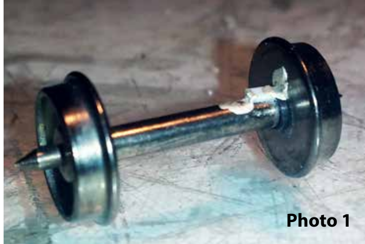
A surface mount technology (SMT) resistor turns a standard Intermountain Railway wheelset into a resistor wheelset.
