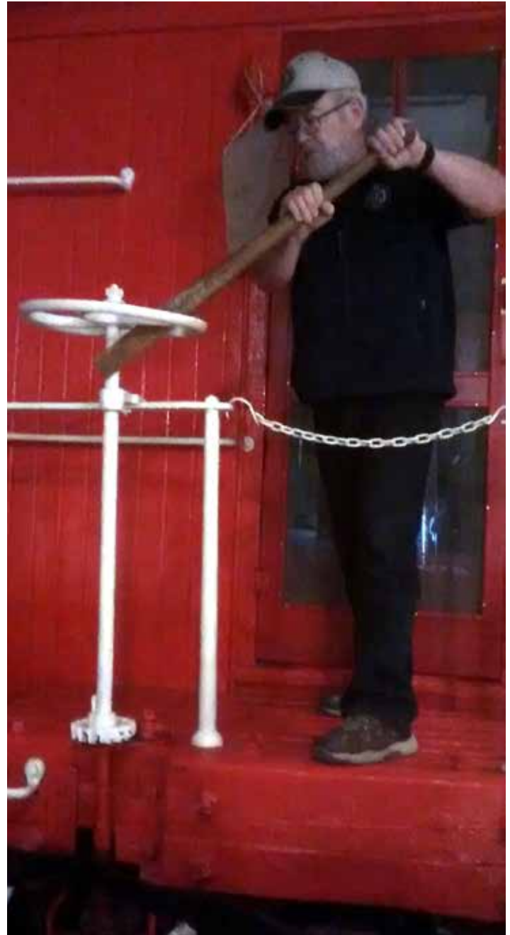
Museum volunteer Rick Inglis demonstrates the use of the Brake Club. Note that one end is squared off to give a better grip against the round brake staff.
